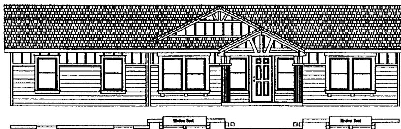
Front View - Exclusive Exterior S 4/12 Roof Pitch - Entry Dormer - Secondary Dormer - Available in Oregon and Washington only Alternate Construction Approval required (AC Letter)
